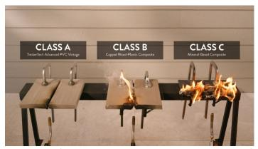
The controlled-environment video features the TimberTech Advanced PVC Vintage Collection, which holds a Class A Flame Spread Rating, and demonstrates its performance under direct flame exposure compared to two competitor decking products with lower flame spread ratings — a Class B capped wood-plastic composite and a Class C mineral-based composite. The results clearly demonstrate TimberTech's Vintage Collection's superior resistance to
